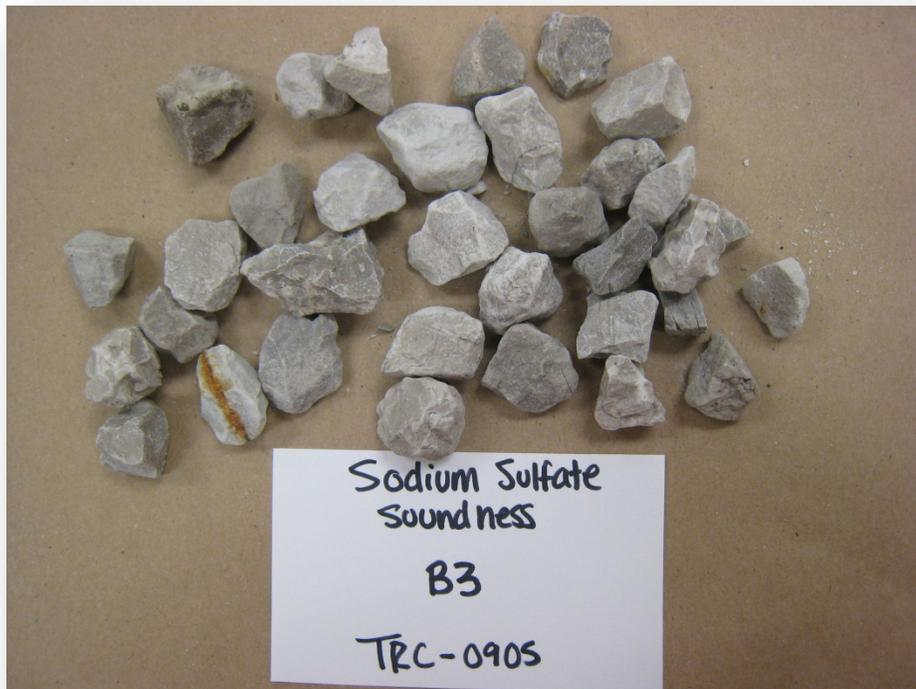
**Figure 10. Aggregates After Testing by the Sulfate Soundness Method (AASHTO T 104)**
