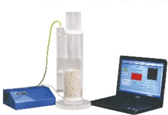
**Figure 13. The SG-9 Aggregate Specific Gravity & Absorption Device**
