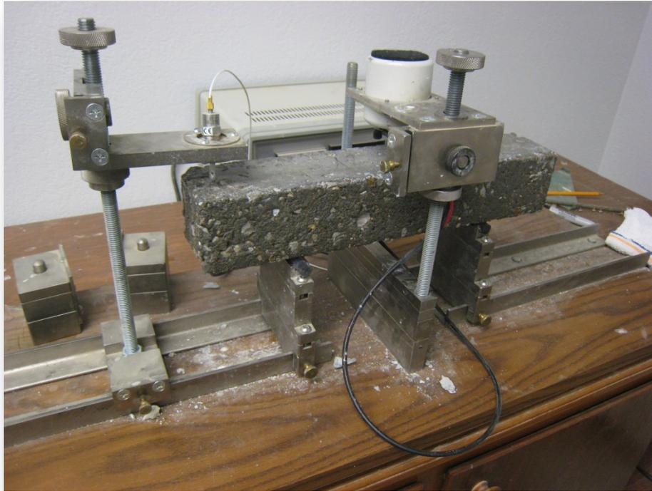
**Figure 7. Measurement of Resonant Frequency**
