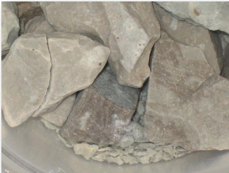
**Figure 12. Aggregates After Testing by the Deep Freeze Method**
