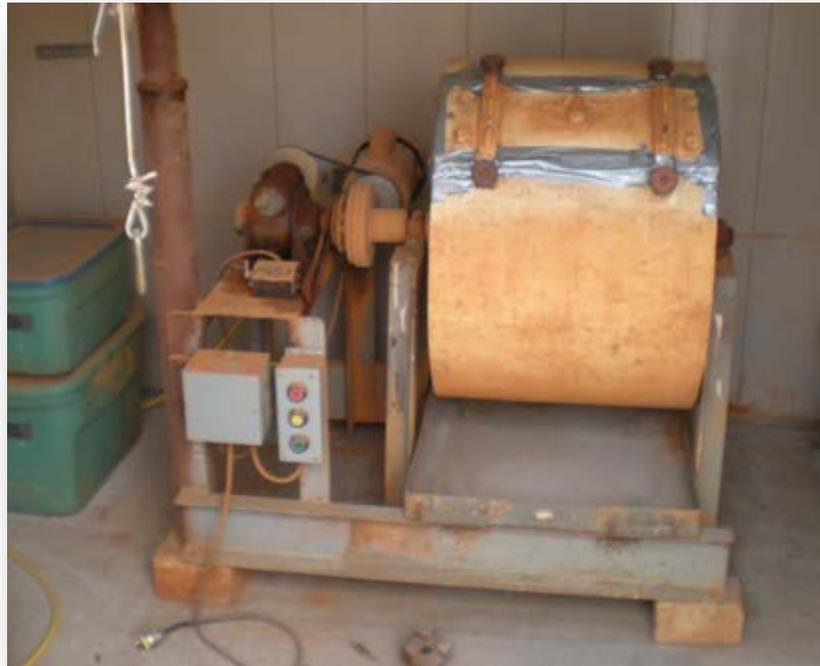
**Figure 1. L.A. Abrasion Machine**
