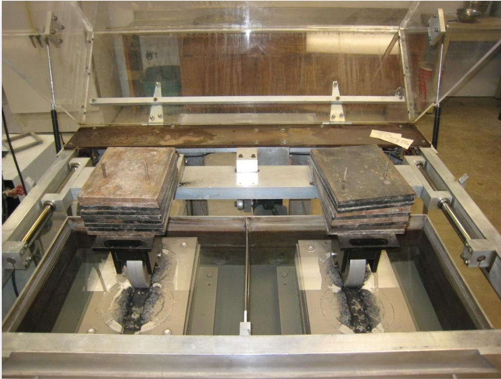
Figure 5. The Evaluator of Rutting and Stripping in Asphalt (ERSA)
