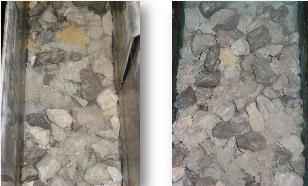
**Figure 11. Aggregates After Testing by the Aggregate Freeze-Thaw Method (AASHTO T 103)**
